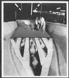
The bottom of your Winner boat is many times tougher and more durable than ordinary boats. That's because the plywood cockpit deck is installed chine-to-chine, and completely encased in protective sealants. On the underside with resin plastic and on top by a thick layer of fiberglass and resin plastic. Thus the planing surface, "grillage" reinforcement and cockpit deck all become one unitized structure - like the frame and body of expensive automobiles.
