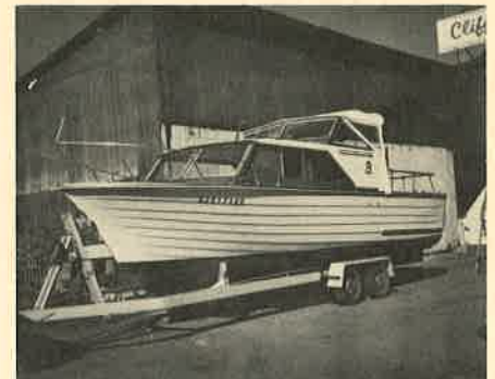
V-hull design, mahogany lapstrake construction
