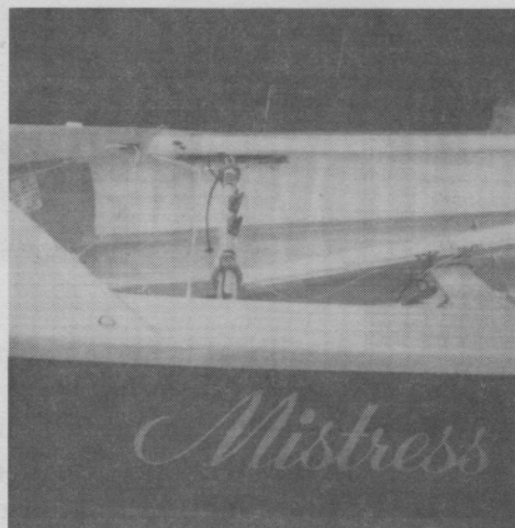
The position of the bar in relation to the shrouds.
