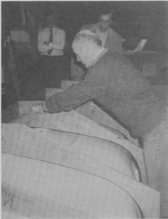
JOHN CHANDLER, FORMER PRINCIPAL OF SKENE INDUSTRIES ASSISTS IN THE PLACEMENT OF THE TEMPLATES USED TO CHECK THE FIRST HULL, WHILE DAVID WEAVER AND COMMODORE CHARLES COLMAN CHECK THE NEW BOAT.
