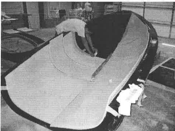
Thermo Formed Foam Core Material in HAPCO Albacore Mold
