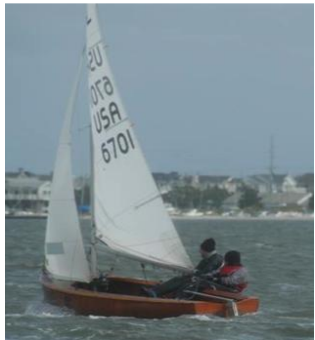
Note top of jib so twisted that its luffing.
