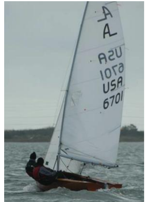
Large mast bend and twisted open leech.
