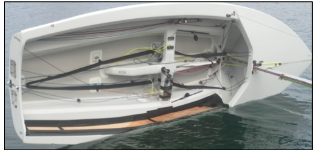
Ovington with additional buoyancy attached, simulating a thicker, more buoyant hull for self-draining.
