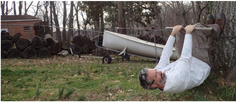
Figure 4. HAPCO Shroud Tensile Proof Test Facility in Operation.
